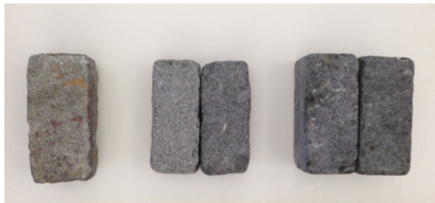
Figure 27: A historic Belgian block from the Gansevoort Market reconstruction project (left), with new, accessible alternatives.
